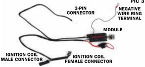
**STEP 6** Refer to PIC 4. Feed the controller's ignition coil connectors wire through an open slot of the frame, under the seat area.
