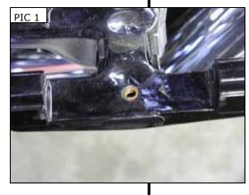
STEP 5 See PIC 1. To help keep the detent ball in place during the installation of the new footboard, place a dab of grease on the hole in the mount that holds the detent ball and spring. Place the detent ball into position as shown in PIC 2.
