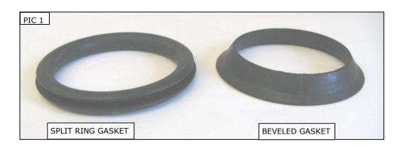
WARNING SOME MOTORCYCLES HAVE HAD THE GAS TANKS REPLACED. MAKE SURE THAT YOU PAY CLOSE ATTENTION TO THE GASKET THAT IS ON THE CAP YOU ARE REPLACING AND USE THE CORRECT REPLACEMENT GASKET. FAILURE TO USE THE CORRECT GASKET MAY RESULT IN FUEL LEAKING AND CREATE A FIRE HAZARD CAUSING LOSS OF CONTROL OF THE MOTORCYCLE. THIS COULD RESULT IN SERIOUS INJURY OR DEATH. PIC 4 AND PIC 5
