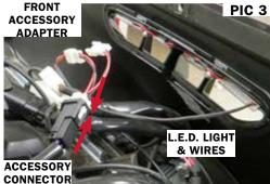
STEP 8 Refer to PIC 4. Locate and insert the male 3-pin connector from the L.E.D. Fairing Vent Light into the female connector of the Front Accessory Adapter.
