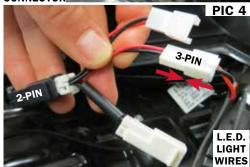
STEP 9 Reinstall the main fuse, turn the ignition on, and test for proper function of the lights. The L.E.D. Fairing Vent Accent is a running light. Turn ignition off.
