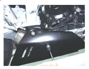
8. For easier dismount of stock muffler, loosen the header tubes (Figure 17) then unscrew the bolts from the headers-collector bracket (Figure 18, 19). Make sure not to damage the cooling fins.
