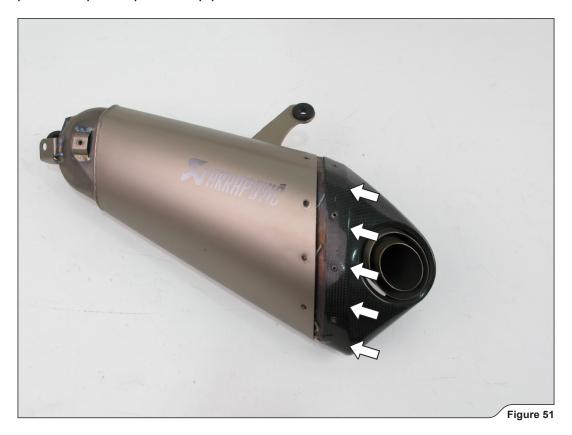
6. Insert the rivets supplied in the Akrapovič reparation kit into the mufflers, as shown (Figure 52).
